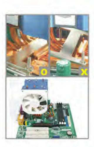
Press the "H" plate with one hand and tighten the nuts to each screws with the other hand. Then, tighten additional nuts to each screws to ensure proper installation.
